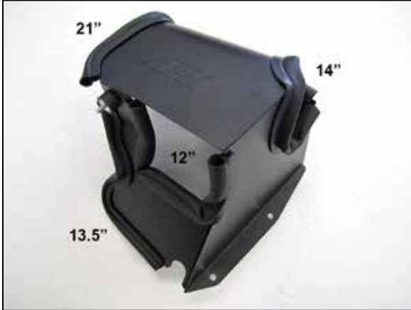
13. Install the edge trim onto the heat shield as shown.
