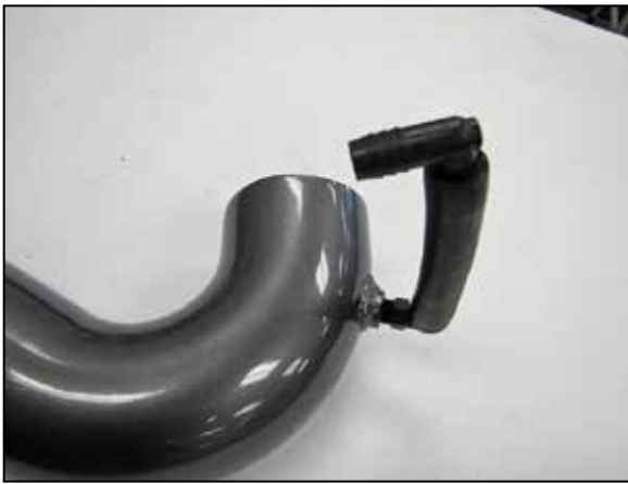
17. Install the provided crank case vent and 90° union fitting onto the AEM® intake tube as shown.
