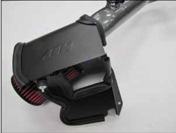
18. Install the AEM® intake tube through the heat shield and install the AEM® air filter onto the tube and secure with the provided hose clamp.
