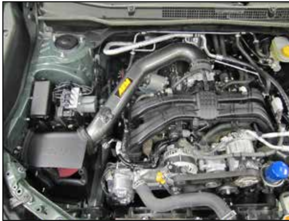
19. Set the intake assembly into the vehicle, using the provided coupler (5-323) secure the intake tube to the throttle body.
