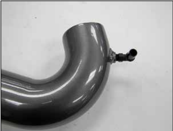
16. Install the 90° vent fitting into the AEM® intake tube as shown. NOTE: Plastic NPT fittings are easy to cross thread. Install the vent fitting “hand” tight, then turn it two complete turns with a wrench.
