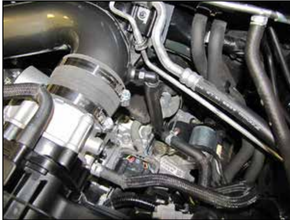
21. Adjust the tube for best fit and then secure with the provided hose clamps.
