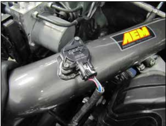
22. Reconnect the mass air sensor electrical connection.
