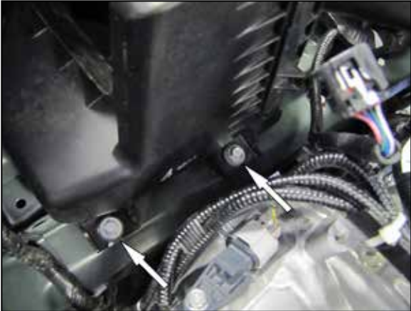
8. Remove the two bolts that secure the factory air filter housing to the frame rail.
