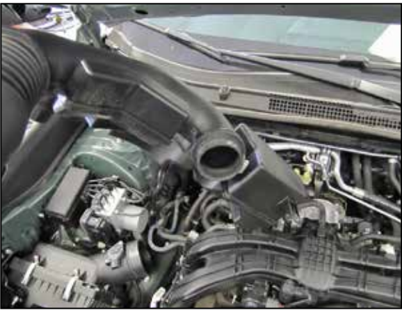
7. Remove the factory intake tube from vehicle.
