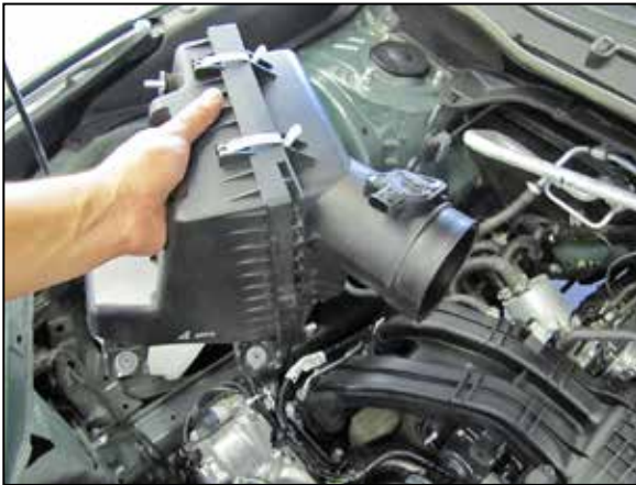
10. Remove the complete air filter housing assembly from the vehicle. NOTE: AEM recommends that customers do not discard factory air intake.
