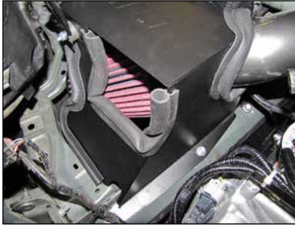
20. Secure the heat shield to the frame rail with the provided hardware.
