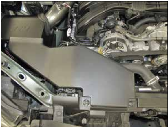
23. Install the fresh air intake duct into the heat shield and then secure with the factory retaining pins.
