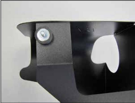
11. Install the rubber mounted stud onto the heat shield as shown.
